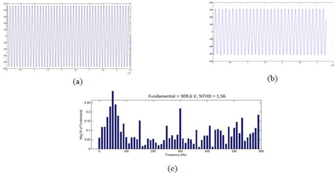
Fig. 3 (a) Transformer input or inverter 1 output (b) Final output or inverter 2 output (c) THDv
