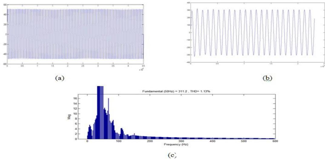
Fig 4 (a) Transformer input or inverter 1 output (b) Final output or inverter 2 output (c) THDv
