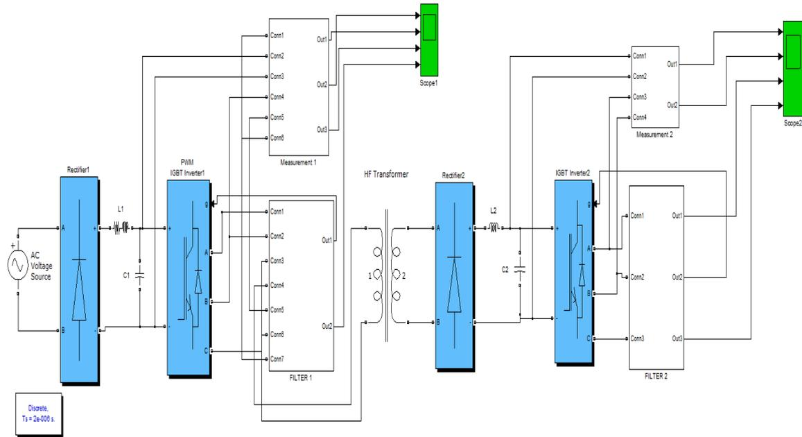
Fig. 2 Simulink model of three stage topology of SST
