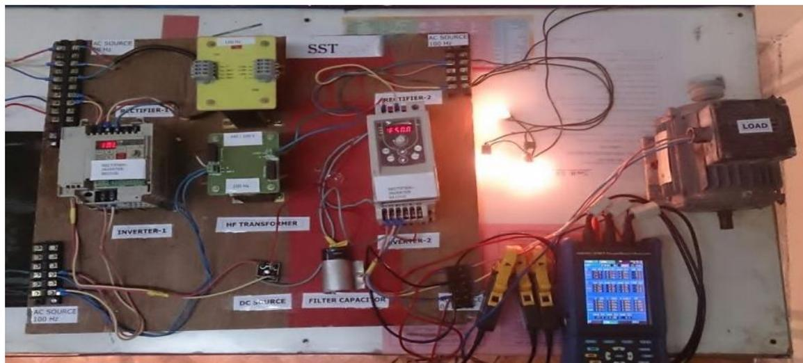
Fig. 5 Hardware model of SST
